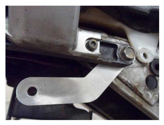
Fit the silencer with clamp on to the link pipe and fit the strap around the silencer and to the bracket with the short spacer.
