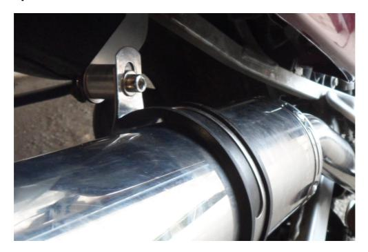
Re-fit footrest bracket bolt using the long spacer.
