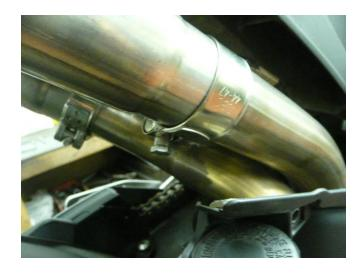
Nip up bolt not too tight for now, just to support it. Smear a light coating of sealant inside silencer and fit with clamp on to link pipe. Now fit strap onto silencer and to frame.
