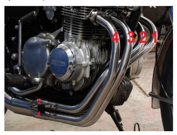
• Fit the brackets onto the silencer.
